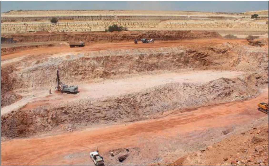
The road grades and width of the permanent ramps, spirals, as well as loading and tipping points, are influenced by the size of the trackless equipment and the effective safe operating slope angle.
